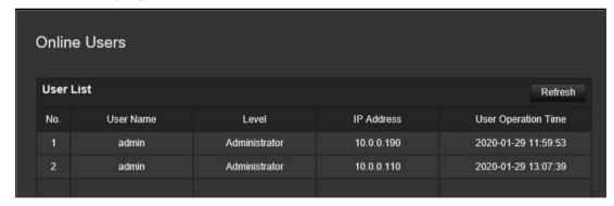
User name, user level, IP address and operation time are displayed. The refresh button reloads the page to check for active connections.
