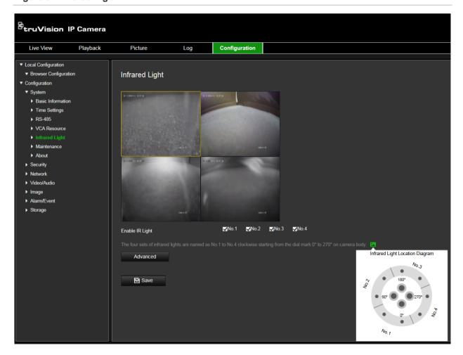
**One-to-One Control:** With one-to-one control enabled, you can bind a certain set of IR LEDs to a specific camera channel. Thus the IR LED only works with the linked camera channel.
