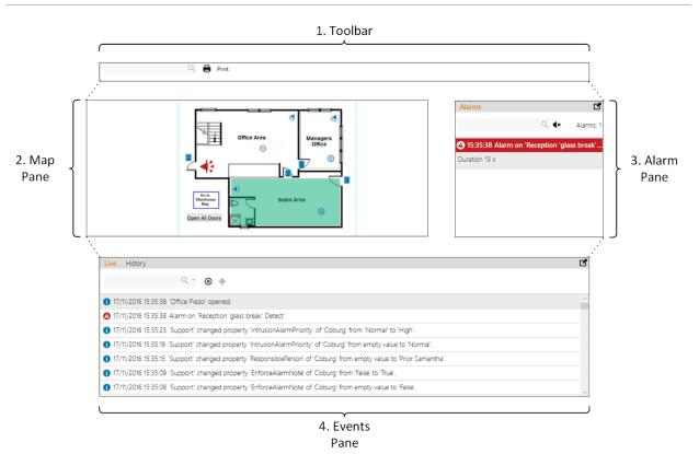
Figure 6: Elements of the Monitor panel
