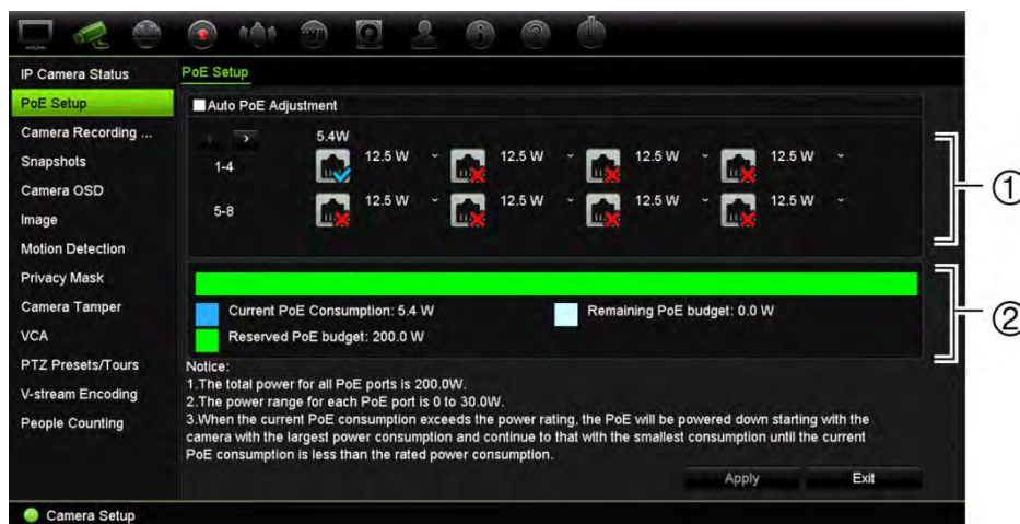
Figure 23: PoE power budget information on IP cameras
