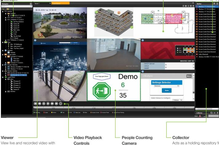
View live and recorded video with up to 10 detachable video viewing tabs allows you to create a virtual video wall. The pop-up event monitor window provides live video during an alarm. Users can easily setup individual video viewing tiles for sequencing of multiple cameras for easy monitoring.
